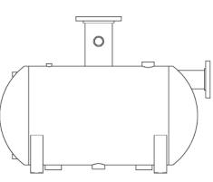
substituted). The trap should be sized with a 3:1 safety factor. If back pressure exceeds tank pressure, the use of a reservoir and pumping trap may be necessary to ensure proper drainage.
